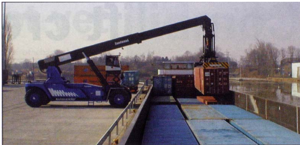
FIGURE 4.1 DOCK-BASED REACH-STACKER OPERATION
