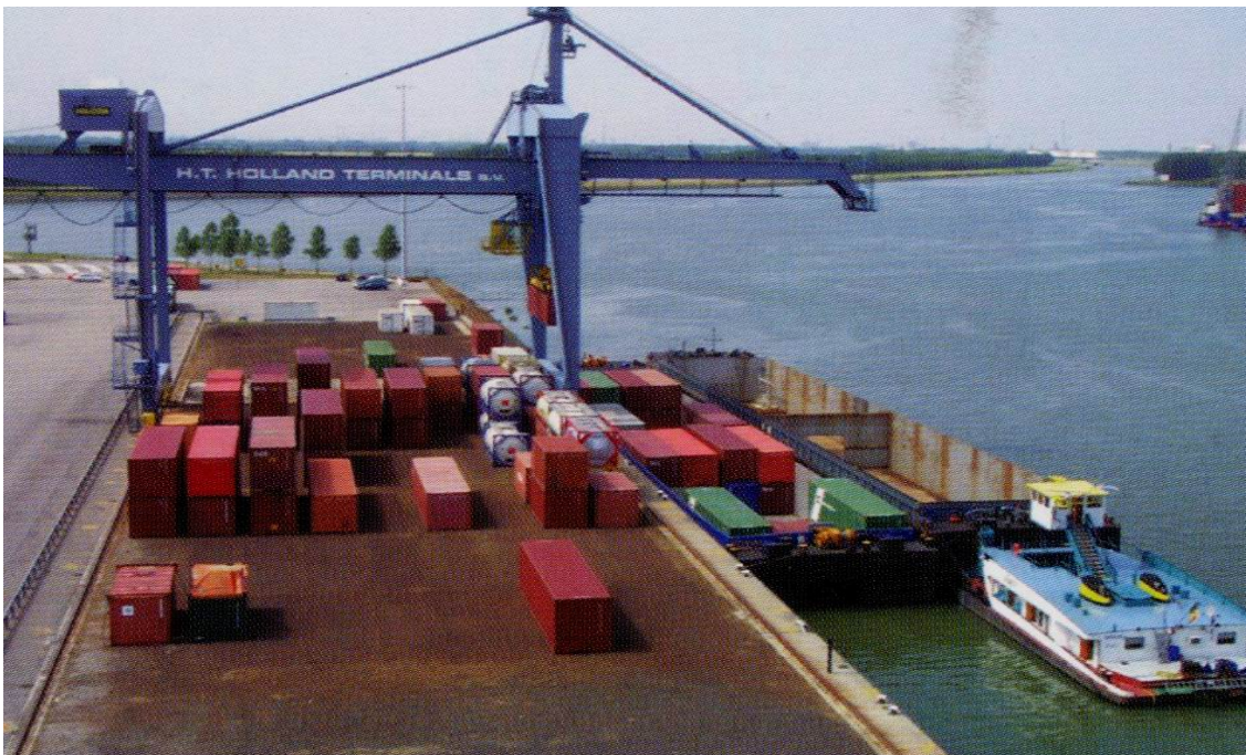
FIGURE 4.4 DEDICATED BARGE-HANDLING RAIL-MOUNTED GANTRY CRANE OPERATION
